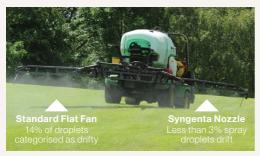
The unique combination of Syngenta's Nozzle design and air induction technology means significantly less drift.
