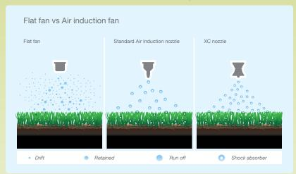
Earlier generation air induction nozzles reduced the drifty component of the droplet spectrum but to achieve this, the penalty was often a reduction in droplets per mL of spray volume. XC nozzles regain the combination of optimal droplet size and number.
